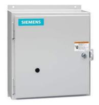
Electrically held lighting contactor, Contactor amp rating 30A, 0 N.C. / 3 N.O. Poles, 347VAC 60HZ coil, Non-combination type, (no disconnect device), Enclosure NEMA type 12, Dust/drip proof for indoors
