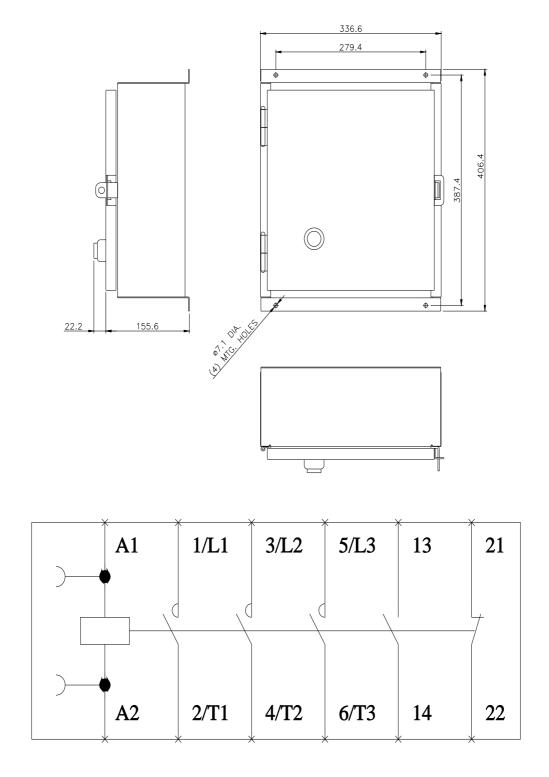
LEN00C003 Wiring Diagram
