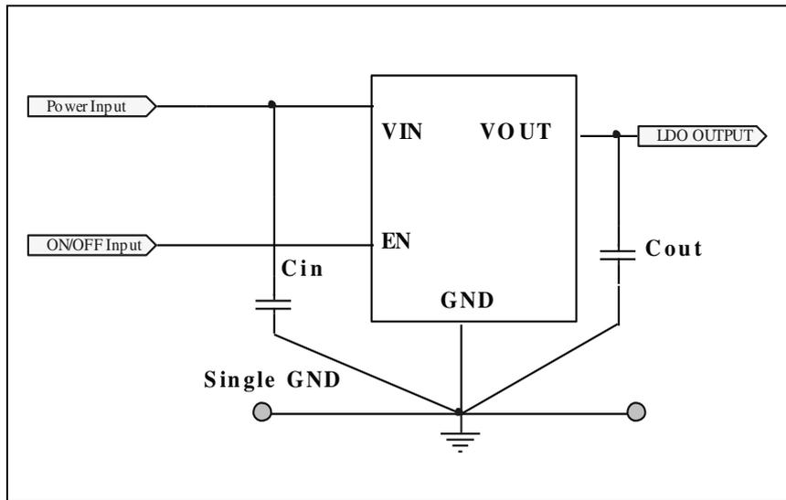
Note:  $C_{in}=C_{out}=1\mu F$
