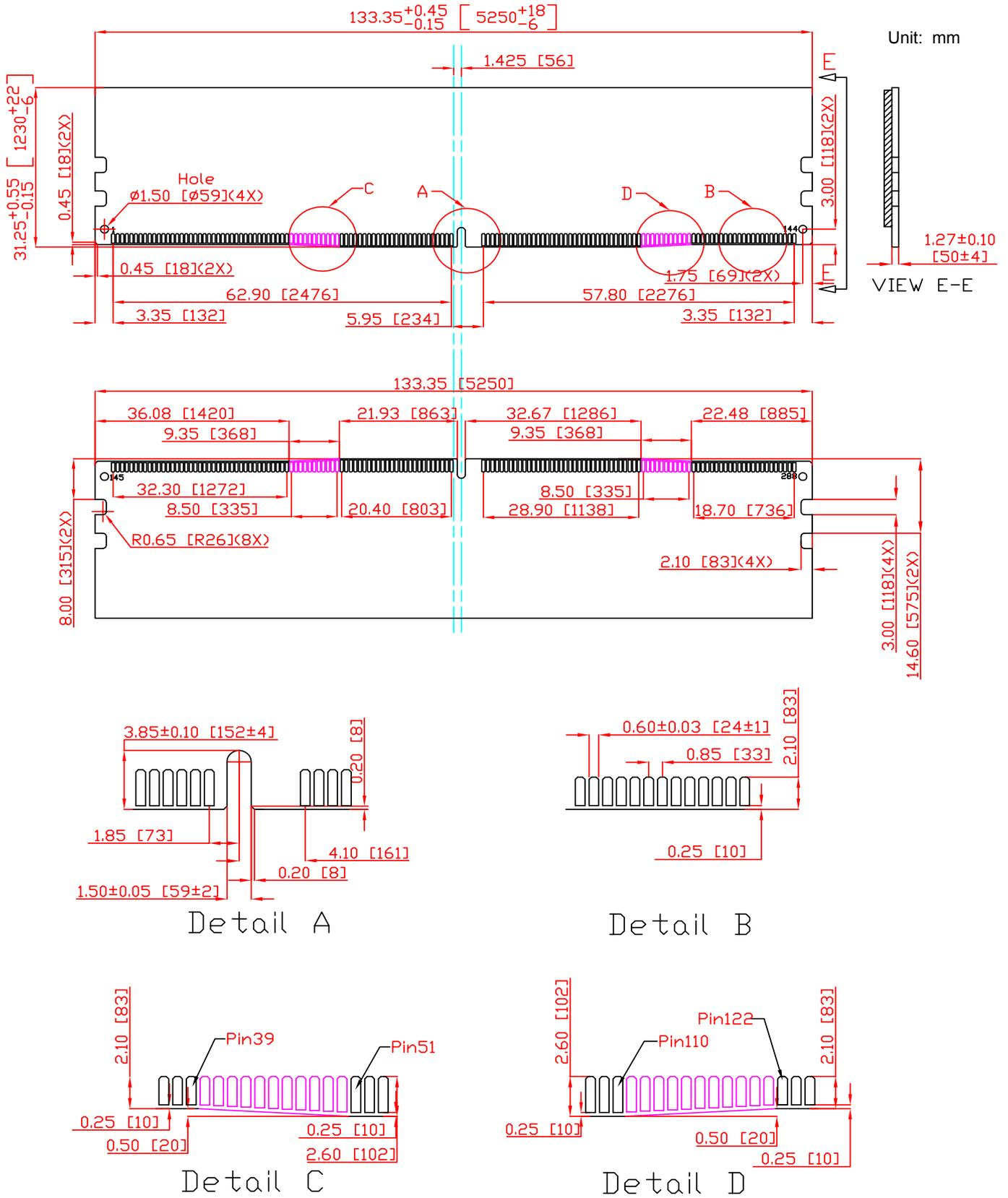
(All dimensions are in millimeters with ±0.15mm tolerance unless specified otherwise.)
