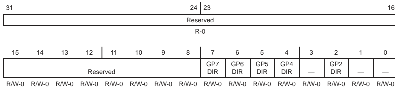
Figure 12. GPIO Direction Register (GPDIR) [Hex Address: 01B0 0004]
