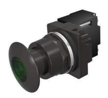
30mm BlackMax, Epoxy Coated Corrosion Resistant Complete Metal Unit Illuminated Push-Pull Operator Transformer type, 120V AC Incandescent Lamp Mushroom Head Cap Small 1 3/4" (44.5 mm) Metal, Black with Green Lens 3 Position Momentary UL Listed, CSA Certified NEMA 1,3,3R,4,4X,12,13 & Automotive Standards
