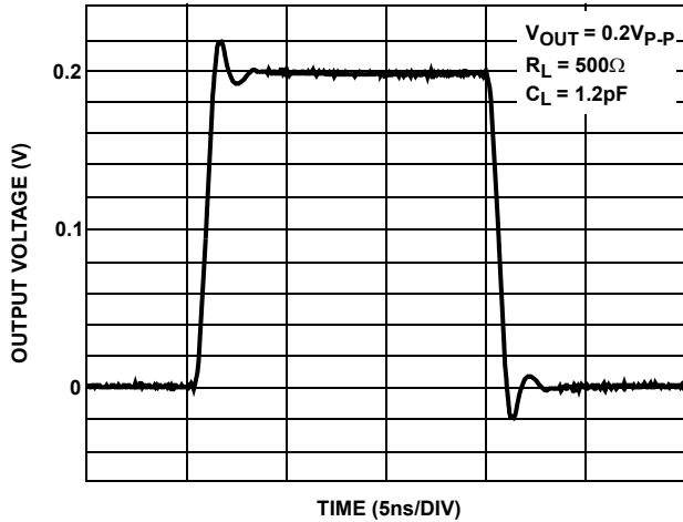
FIGURE 14. SMALL SIGNAL TRANSIENT RESPONSE; R_L = 500\Omega
