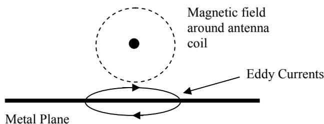
Eddy currents absorb energy and cause detuning of antenna
