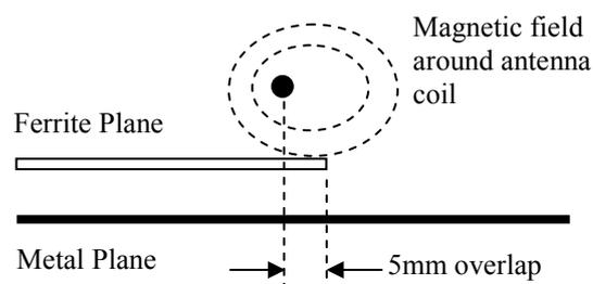
Optimum field distribution, fixed antenna detuning with minimum loss of energy
