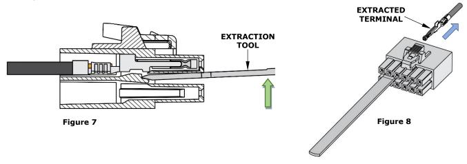
6. Pull the terminated wire out of the connector housing in the direction of the arrow. See Figure 8.
