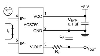
Application 1. The ACS750 outputs an analog signal, V<sub>OUT</sub>. that varies linearly with the uni- or bi-directional AC or DC primary sensed current, I<sub>P</sub>, within the range specified. C<sub>F</sub> is recommended for noise management, with values that depend on the application.
