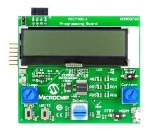
MIC7400/1 Programming Board was designed to demonstrate the MIC7400/1 Power Management IC (PMIC) when programmed by a microcontroller, using an easy-to-understand interface. The board offers increased functionality by the addition of an on-board EEPROM and allows copy, store and also reprogram all the registers in the MIC7400/1 devices
