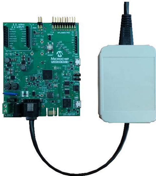
Figure 2-1. PLC-AC-Coupler accessory connected to PL485-EK
