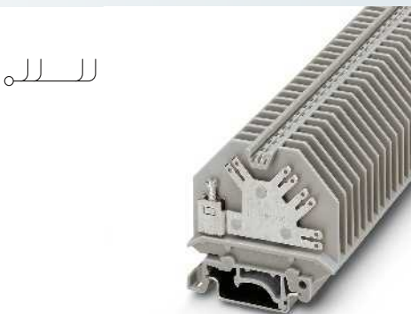
4 (4) mm 2 , 40 A, feed-through terminal block, with screw and spade connection
