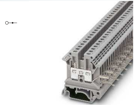
4 (4) mm 2 , 24 A, feed-through terminal block, with screw and solder connection
