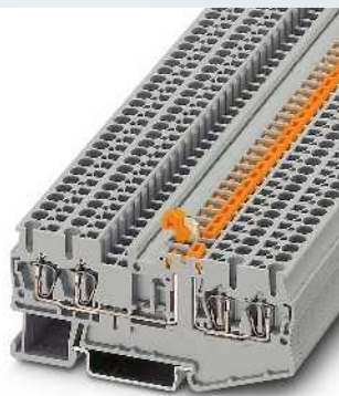
2.5 (4) mm 2 , 20 A, knife disconnect terminal block, 4 connections
