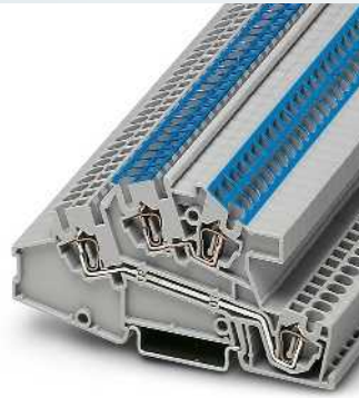
2.5 (4) mm 2 , 24 A, three-level terminal block, 1 x L phase conductor, 1 x N conductor
