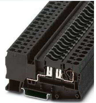
4 (6) mm 2 , 30 A, fuse terminal block for type C flat-type fuses
