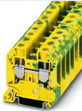
16 (25) mm 2 , 101 A, ground terminal block
