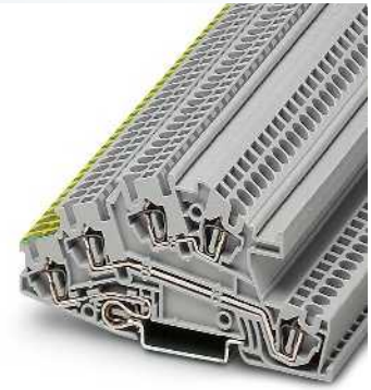
2.5 (4) mm 2 , 24 A, three-level terminal block, 2 x L phase conductor, 1 x PE
