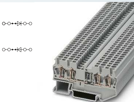
2.5 (4) mm 2 , 0.5 A, diode terminal block, 4 connections
