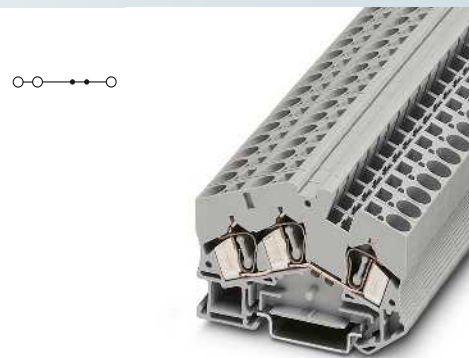
6 (10) mm 2 , 57 A, feed-through terminal block, 3 connections
