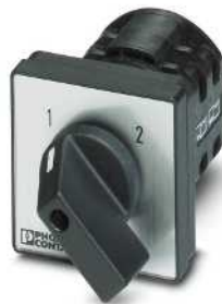
2.5 (2.5) mm 2 , 20 A, changeover switch without 0 position, with electrically isolated contacts
