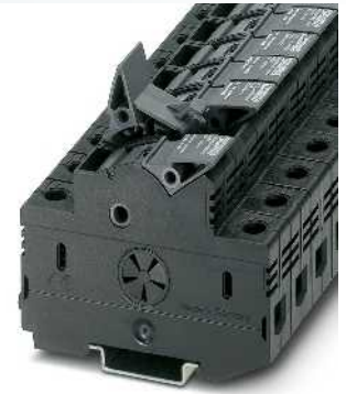
16 (25) mm 2 , 32 A, lever-type fuse terminal block for 10.3 x 38 mm midget fuses
