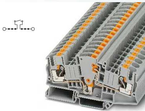
6 (10) mm 2 , 30 A, test disconnect terminal block
