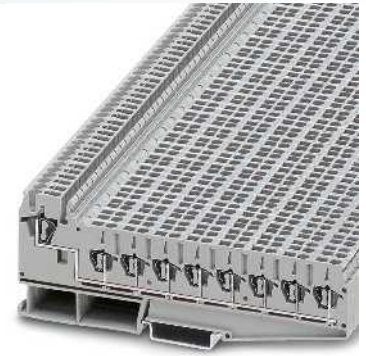
2.5 (4) mm 2 , 24 A, potential distributor terminal block, 8 x 1.5 mm 2 outlets
