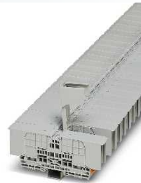
70 (70) mm 2 , 192 A, feed-through terminal block, for DIN rail and direct mounting
