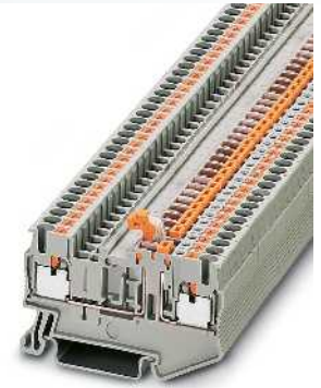
2.5 (4) mm 2 , 20 A, knife disconnect terminal block
