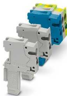
2.5 (4) mm 2 , 24 A, plug, connection at a right angle to the plug-in direction
