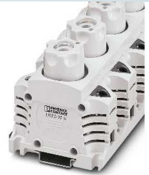
35 (35) mm 2 , 25 A, fuse terminal block for DIAZED D II (E27)
