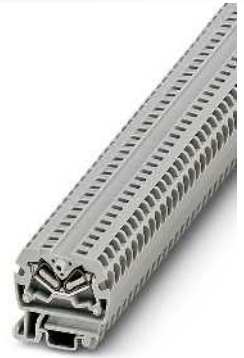
2.5 (4) mm 2 , 30 A, lateral conductor entry, feed-through terminal block
