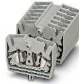
2.5 (4) mm 2 , 30 A, feed-through terminal block, with engagement pin
