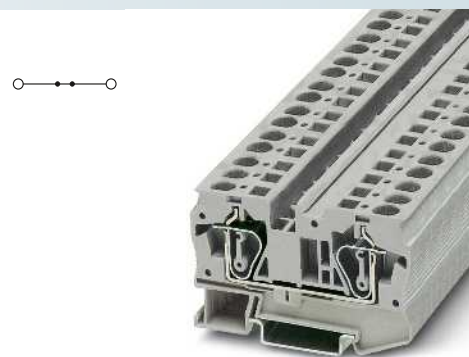
6 (10) mm 2 , 52 A, feed-through terminal block
