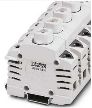
35 (35) mm 2 , 63 A, fuse terminal block for NEOZED D 02 (E18)
