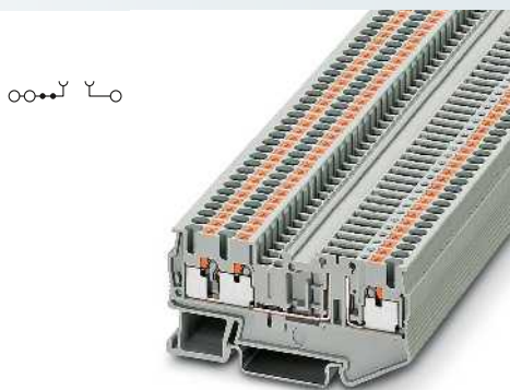
2.5 (4) mm 2 , 20 A, disconnect terminal block, 3 connections
