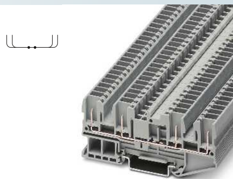
2.5 (4) mm 2 , 24 A, feed-through terminal block, 4 connections
