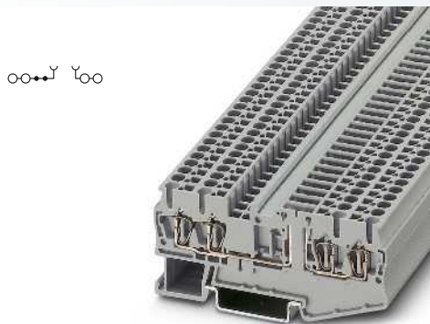
2.5 (4) mm 2 , 20 A, disconnect terminal block, 4 connections
