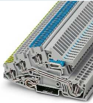
2.5 (4) mm 2 , 20 A, three-level terminal block, 1 x L phase conductor, 1 x N conductor can be disconnected, 1 x PE
