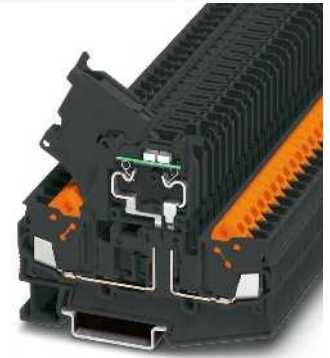
2.5 (2.5) mm 2 , 6.3 A, lever-type fuse terminal block for 5 x 20 mm cartridge fuses
