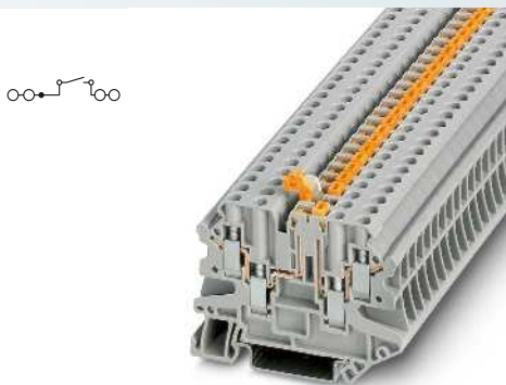
4 (6) mm 2 , 20 A, knife disconnect terminal block, 4 connections
