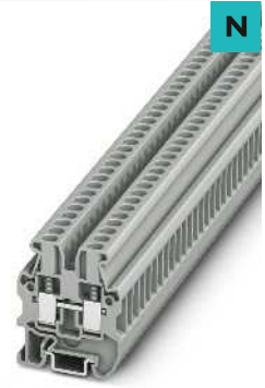
2.5 (4) mm 2 , 32 A, mini feed-through terminal block
