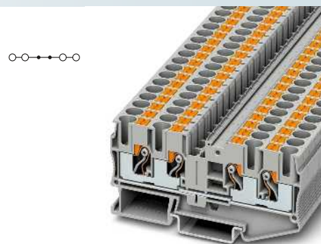
6 (10) mm 2 , 52 A, feed-through terminal block, 4 connections
