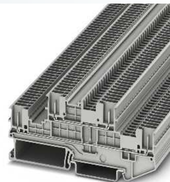
1.5 (1.5) mm 2 , 16 A, double-level terminal block
