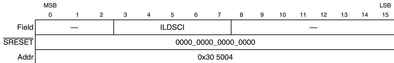
Figure 15-5. QSM2 Dual SCI Interrupt Level Register (QDSCI_IL)
