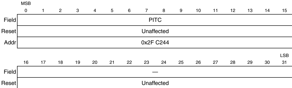
Figure 6-39. Periodic Interrupt Timer Count (PITC)
