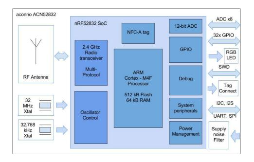
Solely the addition of a suitable DC power source is necessary for BLE and/or ANT connectivity. As a result of its Tag-Connect capabilities, the ease of application is further increased. Sensor applications require additional appropriate sensors.
