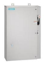
Non-reversing motor starter Size 1 Three phase full voltage Solid-state overload relay OLRelay amp range 3-12A Combination type 30Amp nonfusible disconnect Encl NEMA type 4X 316 S-steel Water/dust tight noncorrosive Extra-wide enclosure
