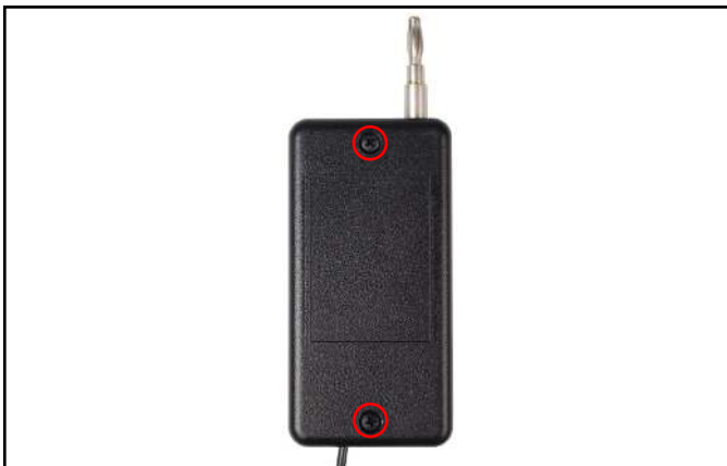
Figure 6. Locating the enclosure screws
