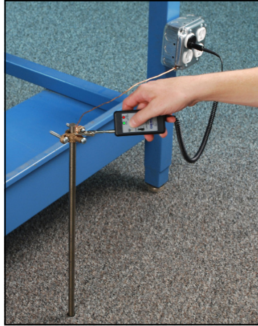
Figure 5. Testing auxiliary ground with the 19249 tester
