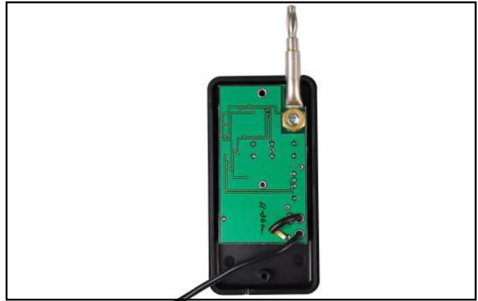
Figure 7. Removing the back cover
