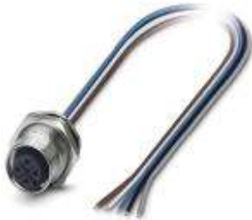
Sensor/actuator flush-type socket, 5-pos., M12 SPEEDCON, A-coded, rear/screw mounting with Pg9 thread, with 0.5 m TPE litz wire, 5 x 0.34 mm 2
