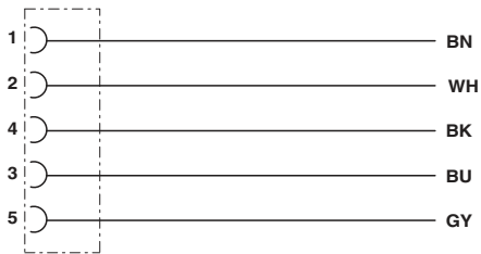
Contact assignment of the M12 socket
