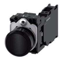
Pushbutton, 22 mm, round, plastic, black, pushbutton, flat, momentary contact type, with holder 1 NO+1 NC, spring-type terminal,
