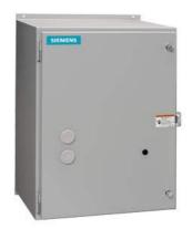
Mechanically held lighting contactor, Contactor amp rating 200Amp 0NC  $\_$  5NO poles, 110VAC 50HZ/120VAC 60HZ coil, Non-combination type, Encl NEMA type 4X 304 S-steel Water/dust tight noncorrosive
