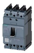
circuit breaker 3VA5 UL frame 125 breaking capacity class S 25kA @ 480V 3-pole, line protection TM210, FTFM, In=100A overload protection Ir=100A fixed short-circuit protection Ii=10 x In UL 489 SB (naval), 50° C without connection
