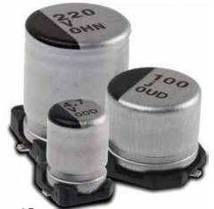
Type AVEK Capacitors are rated for 5000 hours at 105 °C with low impedance characteristics. They are ideal for high density PC board packaging. The Type AVEK offers a low in-place-cost for a high quality performer. The vertical cylindrical cases facilitate automatic mounting and reflow soldering into the same footprint of like-rated tantalum capacitors except without the need for voltage derating. Type AVEK is RoHS compliant.
