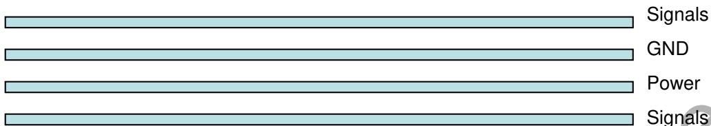
Figure 29: Typical 4-layer PCB construction
