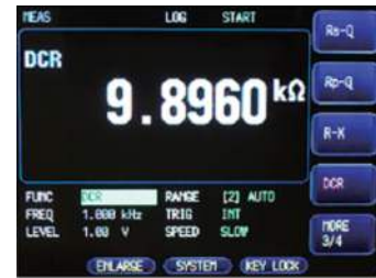
D.C. Resistance Measurement Ideal for inductive components' D.C. Characteristics Verification
