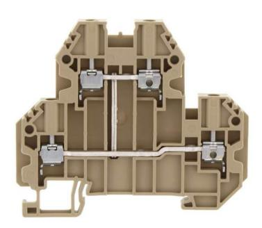
Double-level terminal, Screw connection, Mounting type: Mounting rail TS 35/7.5, Rated cross-section: 2.5 mm², Width: 5.1 mm, Colour: Beige
