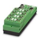
The stand-alone device for CANopen<sup>®</sup> has 16 digital inputs. The M12 connection is established using fast connection technology. The 24 V DC supply is protected against short circuit and overload. The nominal current of the device is 1.2 A.
