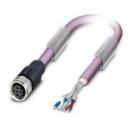
Bus system cable, CANopen $^{\otimes}$ , DeviceNet $^{\text{TM}}$ , 5-position halogen-free, shielded, free cable end, on Socket straight M12, coding: A, cable length: 5 m
