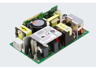
Advanced Energy's Artesyn LPS200-M series medically-approved AC-DC power supplies are available with a nominal main output of 5 V, 12 V, 15 V, 24 V or 48V. Auxiliary 12 V fan output is also provided. LPS200-M power supplies provide 125 Watts of output power with free air convection cooling or up to 250 Watts with 30 CFM of forced air. All models have a power factor of 0.99 typical and a  $3 \times 5 \times 1.32$  inch form factor.
