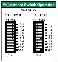
Add the value of switches in the ON position for the total time delay.
