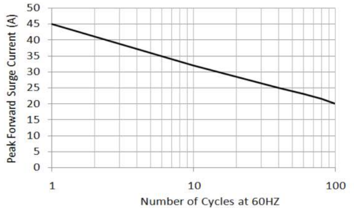
Figure 2. Maximum Non-repetitive Peak Forward Surge Current
