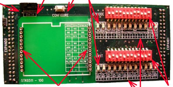
Onboard ATMega8515 uC with preset firmware controls the configuring of the register with the values selected by the DIP switches
