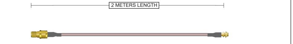
Connector A 132279 SMA Jack Straight Brass Gold + Heatshrink 50 Ohm RG-178 Continuity/Hi-Pot Connector B 262120 MMCX Jack Straight Bulkhead - Rear Mount Brass Gold + Heatshrink
