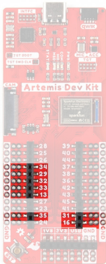
Analog input pins on the Artemis Development Kit. (Click to enlarge)
