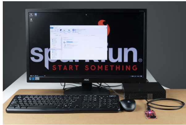
The Artemis Development Kit attached to a computer. The board appears as a mass storage device, named ARTEMIS , in the displayed window. (Click to enlarge)
