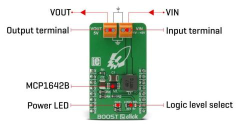
The MCP1642B-ADJ step-up regulator actively damps the oscillations typically found at the switch node of a boost converter. This removes the high-frequency radiated noise, ensuring low noise operation.
