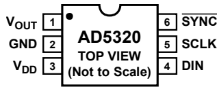
Figure 3. SOT-23 Pin Configuration
