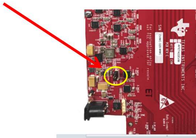
Figure 6. Location of Jumper J9 Circled in Yellow
