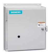
Mechanically held lighting contactor, Contactor amp rating 60Amp 0NC \_ 6NO poles, 440VAC 50HZ/480VAC 60HZ coil, Non-combination type, Enclosure NEMA type 1, Indoor general purpose use
