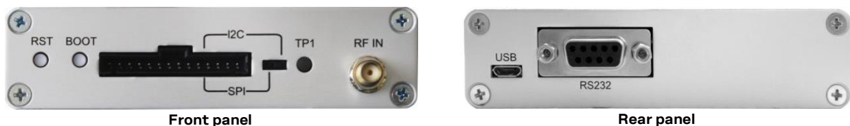
Figure 2: EVK-M8U evaluation unit – front and rear panels
