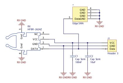
\* Edge SMA connector not assembled.
