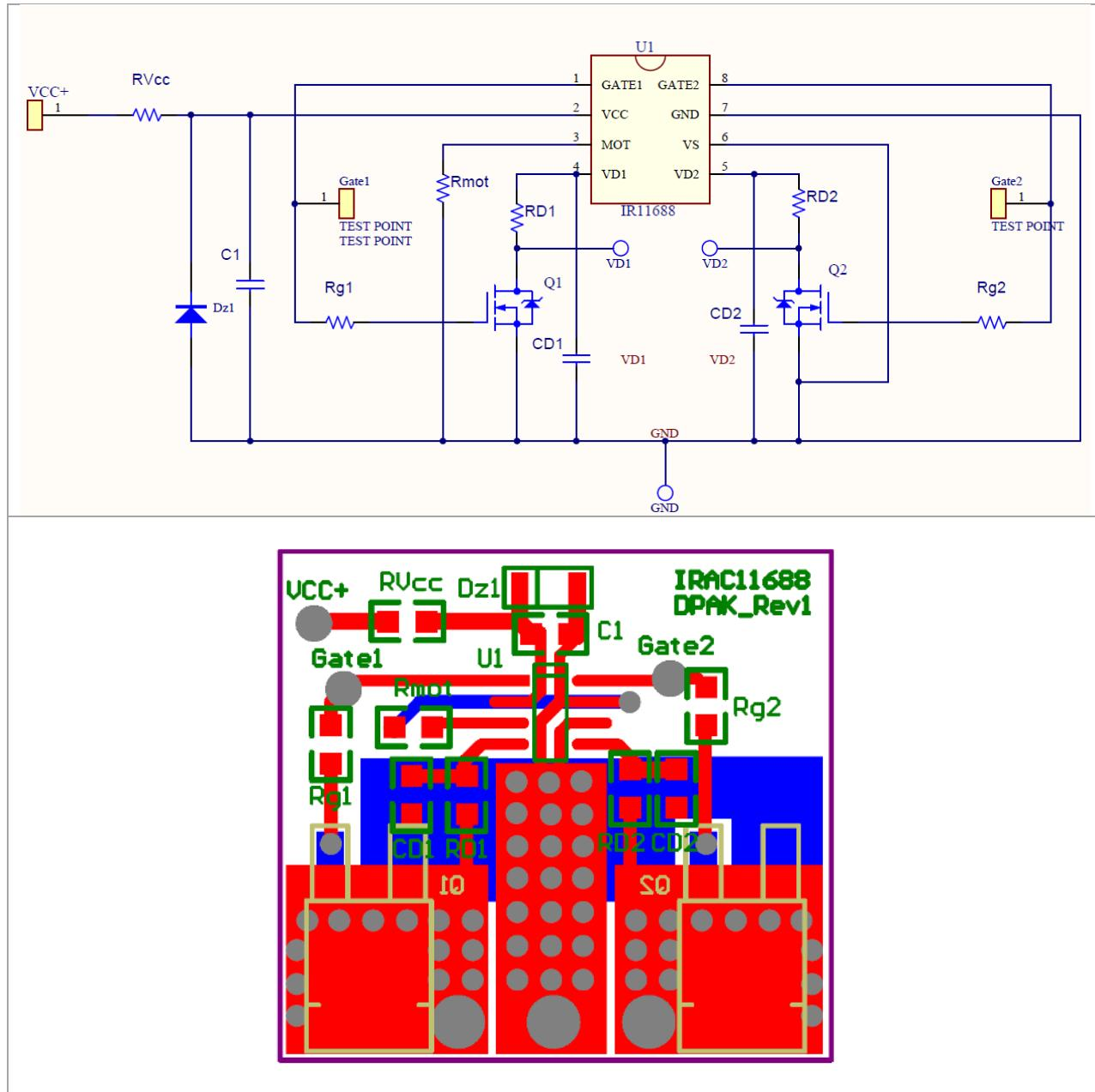
The daughter card shown above is designed to allow easy retrofit in existing systems with minimal system changes. The component values are recommended but user has freedom to change them per application requirement.
