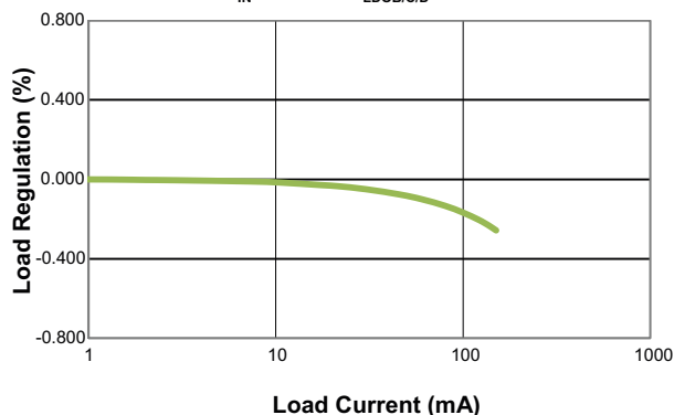
LDOB/C/D Output Voltage Load Regulation (V IN = 3.6V, V LDOB/C/D = 1.2V)
