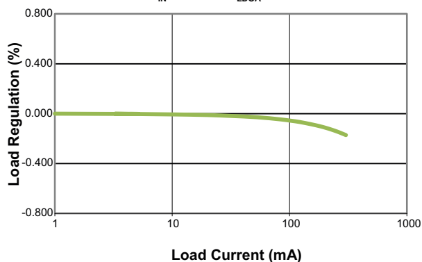
LDOA Output Voltage Load Regulation (V IN = 3.6V, V LDOA = 3.3V)
