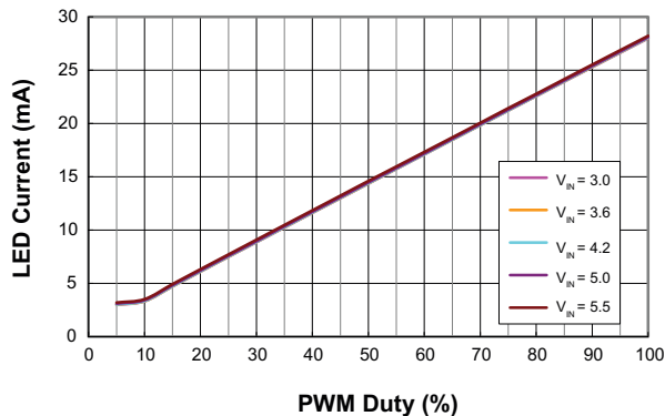
PWM Duty vs LED Current (AAT2893-2 10 WLEDs)
