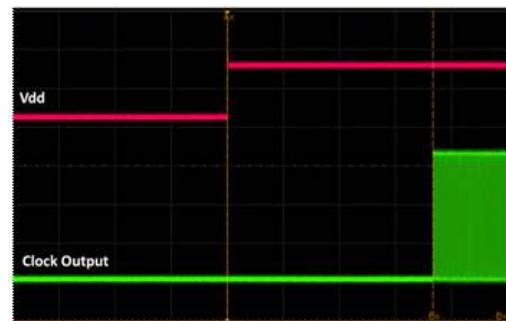
Figure 16. Startup Waveform vs. Vdd
