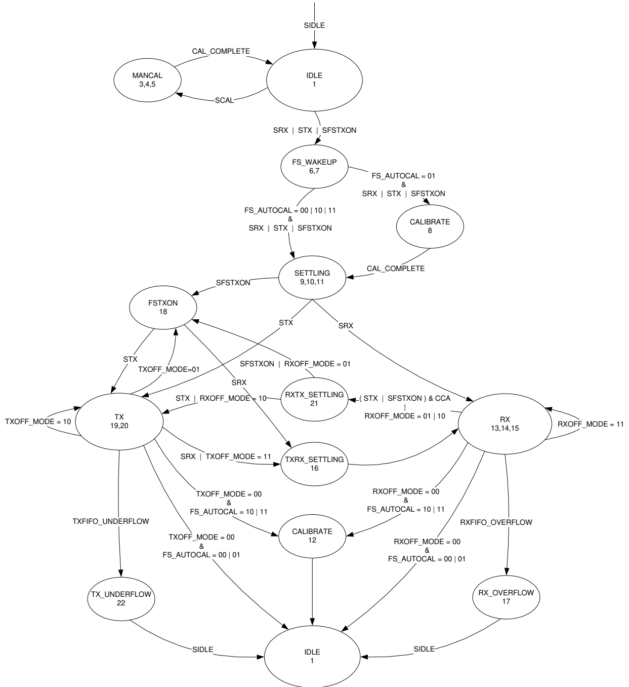
Figure 55: Complete Radio Control State Diagram
