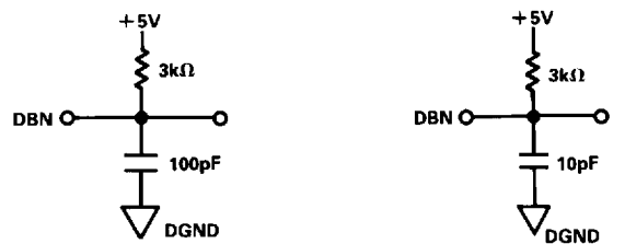
Figure 5. Load Circuit for \overline{INT} Propagation Delays
