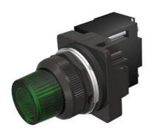
30mm BlackMax, Epoxy Coated Corrosion Resistant Complete Metal Unit Illuminated Indicator Light Full Voltage type, 120V AC/DC Incandescent Lamp, BA9s Glass Lens, Green UL Listed, CSA Certified NEMA 1,3,3R,4,4X,12,13 & Automotive Standards
