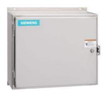
Mechanically held lighting contactor, Contactor amp rating 30Amp 0NC  $\_$  8NO poles, 208VAC 60HZ coil, Non-combination type, Enclosure NEMA type 12, Dust/drip proof for indoors
