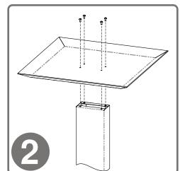
Use Phillips screwdriver to secure base to column with (4x) screws (10-32 x 5/16").
