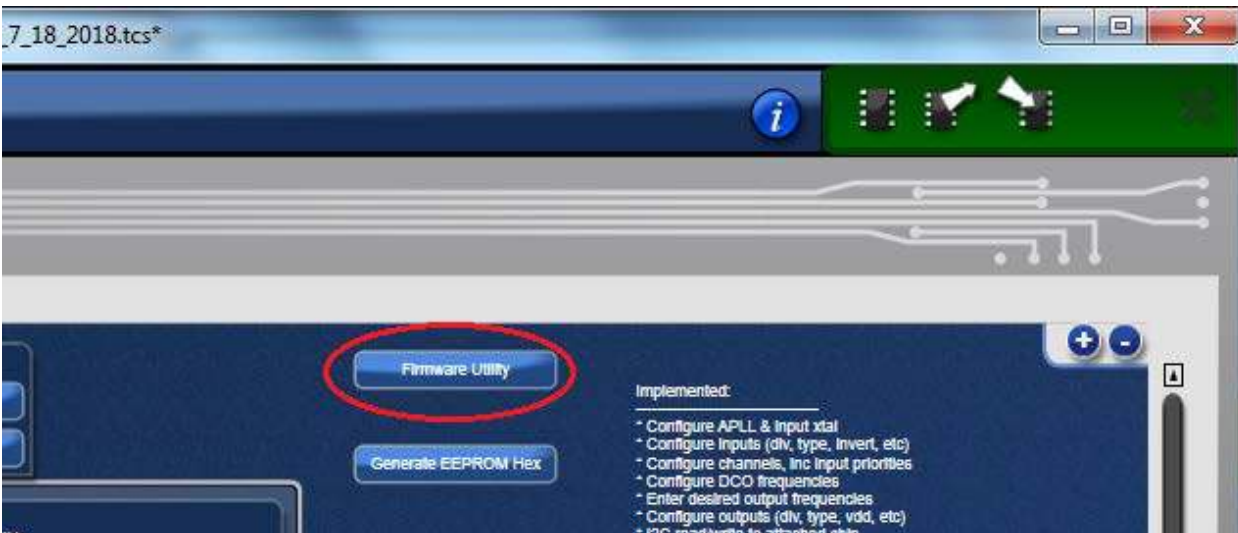
Figure 11. Reading Firmware Version
