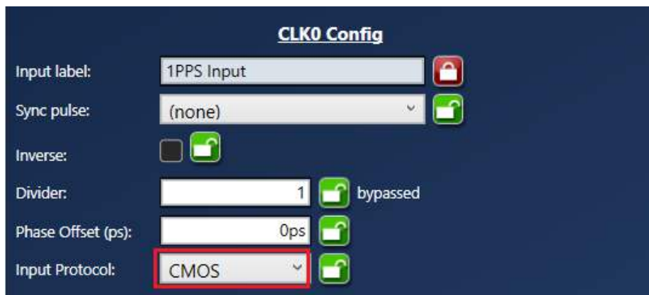
Figure 14. Configuring CLK0 as CMOS to Receive a 1PPS Input
