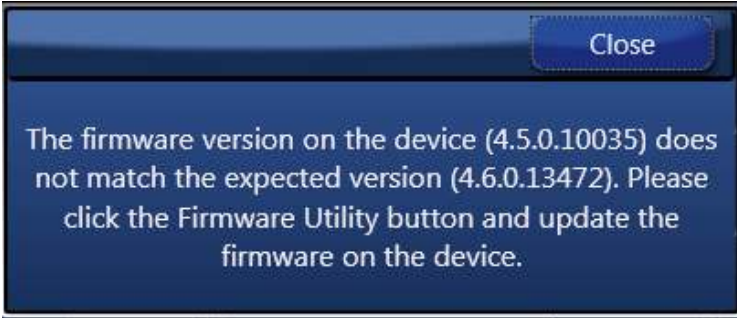
Figure 10. Firmware Version Mismatch Warning Message
