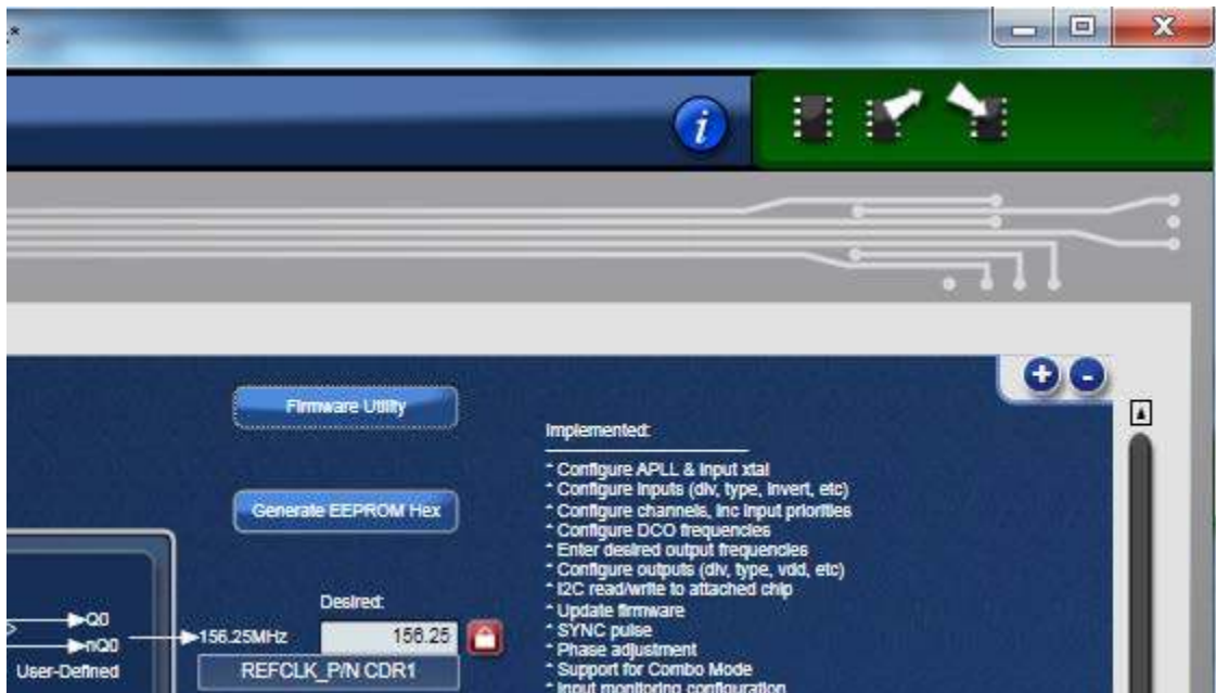
Figure 9. A Green Band appears when a Valid Connection is Made
