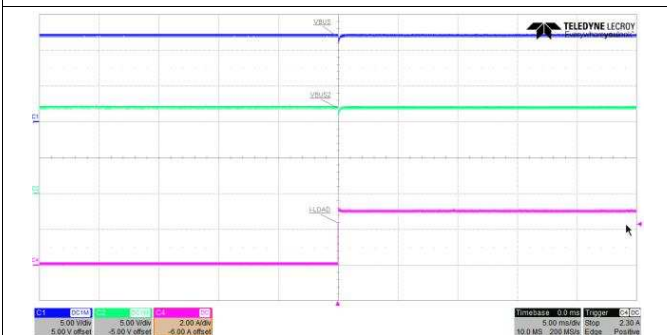
Figure 22. VCONN With 200-mA Load
