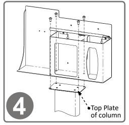
Attach the RS005-0223 Respiratory Hygiene Station to the column using (4x) screws included with stand. Tighten.
