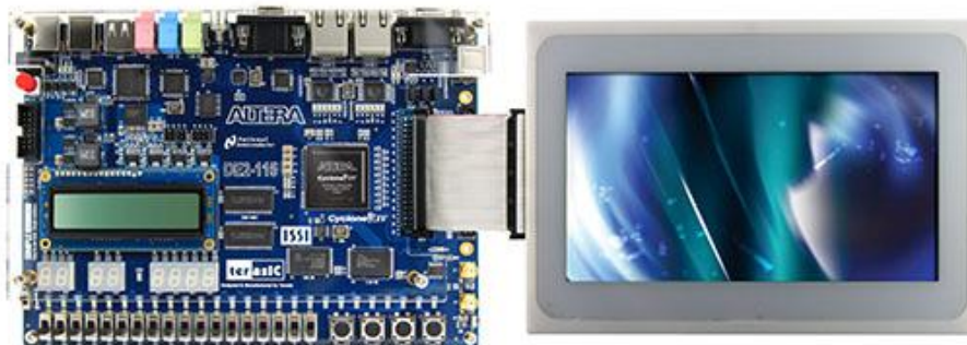
Figure 5-4 Hardware Setup with DE2-115
