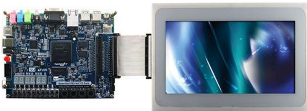
Figure 1-7 MTL2 with DE1-SoC
