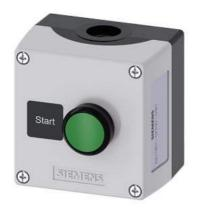
enclosure for command devices, 22 mm, round, enclosure material plastic, enclosure top part gray, 1 control point plastic, recess for label, A=Pushbutton green, label: start, 1 NO, 1 NC, screw terminal, floor mounting, Label glued in
